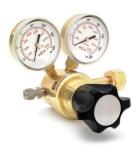
Before using cylinders, read all label information and Safety Data Sheets (SDSs) associated with the gas being used. The cylinder valve outlet connections are designed to prevent mixing of incompatible gases. The outlet threads vary in diameter; some are internal and some are external; some are right-handed and some are left-handed. Generally, right-handed threads are used for fuel gases.
