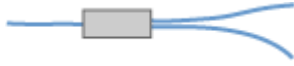
Figure: A fiber-optic beam splitter with a single input port and two output ports.
