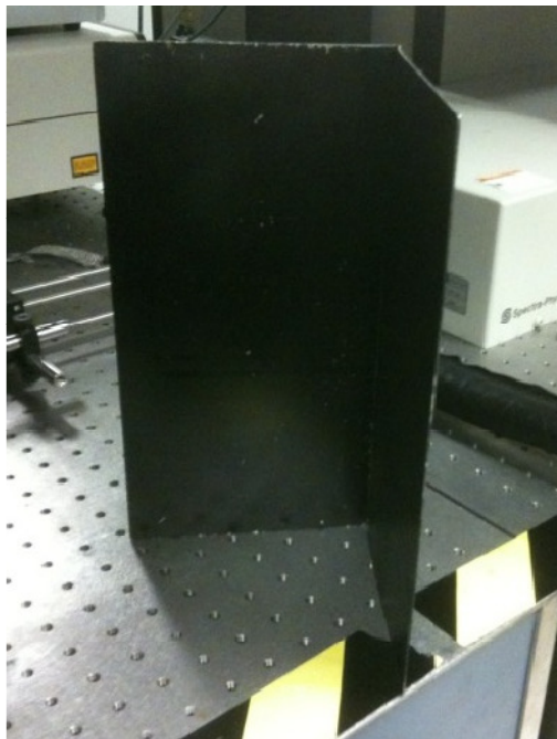
Figure: Unsecured beam block perched on the edge of a laser table
