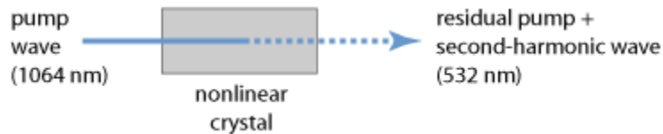
Figure: A typical configuration for frequency doubling: an infrared input beam at 1064 nm generates a green 532-nm wave during its path through a nonlinear crystal.
