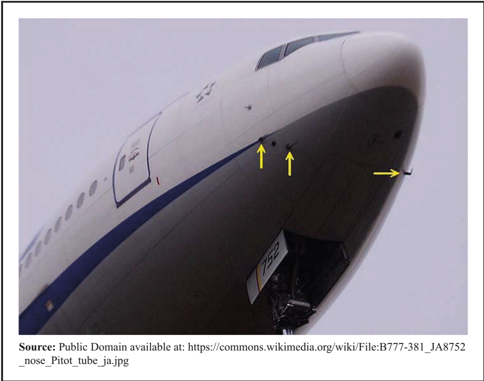
Figure E3 Pitot tube location
